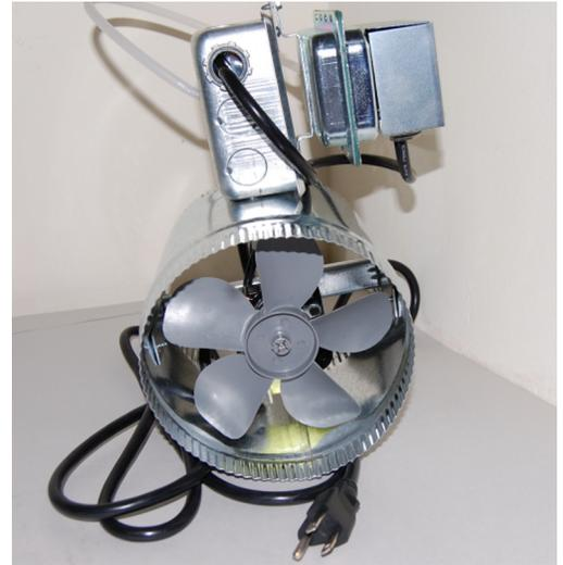
1. To install separate a joint in a branch duct. Cut off a length of duct 1 inch shorter than the duct fan being installed leaving 2 female ends to accept the duct fan. Both ends of Acme Miami duct fans are crimped. Seal both joints with Duct Tape. See Figure 1.
